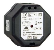
The BL-201 EnOcean-DALI-Gateway provides one DALI master with an integrated DALI power supply for the direct connection of up to 10 slaves (lout max.= 20 mA), without a separate DALI power supply. Also an EnOcean wireless transceiver is integrated. This allows the smart and easy integration and combination of DALI ballasts and EnOcean wireless technology. The BL-201 is supplied by 230 V AC line voltage.
