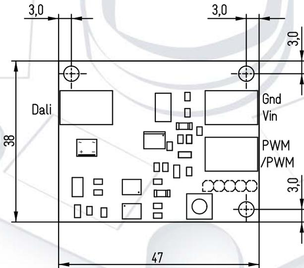
The LED-Warrior07-01MOD generates a PWM signal to control LED drivers. LEDs may not be driven direct by LED-Warrior07-01MOD, an appropriate driver is necessary.
