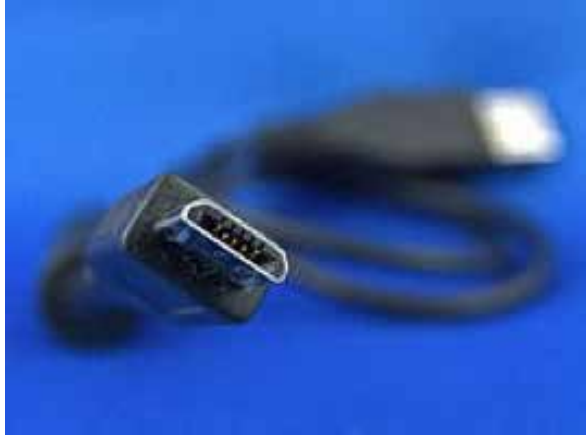
Figure 49: Micro-B USB male cable
