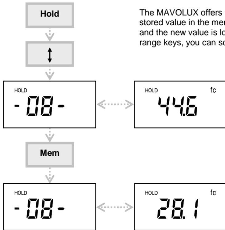
The MAVOLUX offers the function „Mem Edit“ for correcting a stored value in the memory. Measure again, press the **Hold** key and the new value is logged in. Then, by pressing one of the range keys, you can scroll through the memory.
