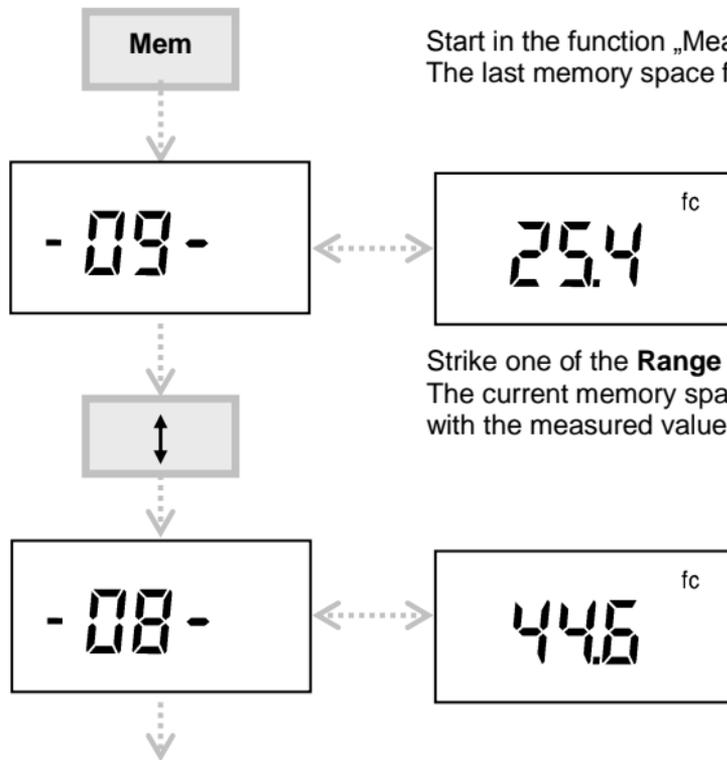
Start in the function „Measuring“ and press down the key **Mem**. The last memory space filled will be displayed first.
