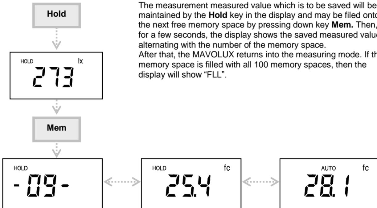
The measurement measured value which is to be saved will be maintained by the **Hold** key in the display and may be filed onto the next free memory space by pressing down key **Mem**. Then, for a few seconds, the display shows the saved measured value alternating with the number of the memory space. After that, the MAVOLUX returns into the measuring mode. If the memory space is filled with all 100 memory spaces, then the display will show “FLL”.
