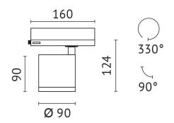
quantity lamps: 1 Light up with: COB LED System power: 25 W Luminous flux: 3198 lm colour temperature: 3000 K colour rendering index: >90
