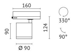
quantity lamps: 1 Light up with: COB LED System power: 25 W Luminous flux: 3134 lm colour temperature: 2700 K colour rendering index: >90
