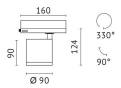
quantity lamps: 1 Light up with: COB LED System power: 25 W Luminous flux: 3266 lm colour temperature: 3500 K colour rendering index: >90
