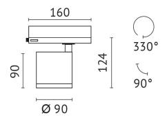
quantity lamps: 1 Light up with: COB LED System power: 25 W Luminous flux: 3299 lm colour temperature: 4000 K colour rendering index: >90
