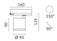
quantity lamps: 1 Light up with: COB LED System power: 25 W Luminous flux: 3169 lm colour temperature: 2700 K colour rendering index: >90
