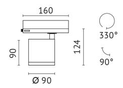
quantity lamps: 1 Light up with: COB LED System power: 25 W Luminous flux: 3102 lm colour temperature: 2700 K colour rendering index: >90
