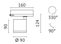
quantity lamps: 1 Light up with: COB LED System power: 25 W Luminous flux: 3263 Im colour temperature: 4000 K colour rendering index: >90
