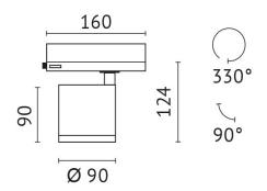
quantity lamps: 1 Light up with: COB LED System power: 25 W Luminous flux: 3234 lm colour temperature: 3000 K colour rendering index: >90
