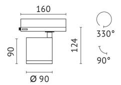
quantity lamps: 1 Light up with: COB LED System power: 25 W Luminous flux: 3229 lm colour temperature: 4000 K colour rendering index: >90
