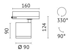
quantity lamps: 1 Light up with: COB LED System power: 25 W Luminous flux: 3230 lm colour temperature: 3500 K colour rendering index: >90
