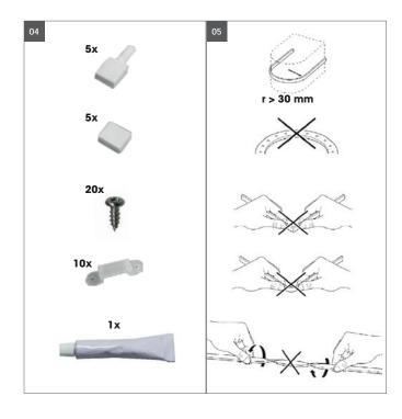
**04.** Minimum radius of bending 30 mm. **Do not bend**, bending will damage the conductors. Do not install below 0°C or bend the LED band.
