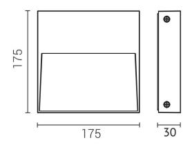
Light up with: LED System power: 10 W Luminous flux: 800 lm
