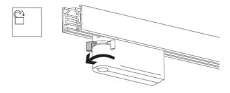
In the second step, set up the electrical connections by turning the second rocker lever into the locked position, as shown below.
