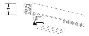
When the installation is done, switch on the light rails power supply, according to the installation and mounting instructions of the manufacturer. The BL-201-12-868 ERCO FLEX is fully functional within a few seconds.
