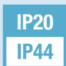
Only when the product is installed in a closed ceiling it may be exposed to water splashes, and only on its front side.
