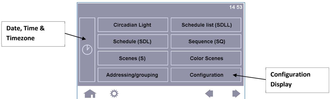
The menu "Configuration" and the button with the clock-symbol refer to display and layout related settings, whereas the other menus are either used for commissioning or for activating functions. Please find a overview of the display-related settings below.
