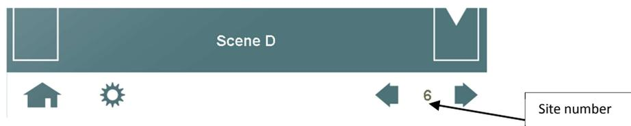
If the site number is pressed for more than 2 seconds it starts flashing. In this state it can be rearranged by using the arrows. By pressing the flashing number for 2 seconds the edit-mode is finished. After arrangement of the sites is finished, displaying the site order can be disabled.
