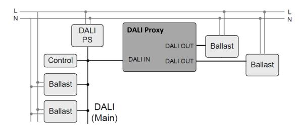
Expansion of a DALI line (Main) with a DALI Proxy (all control commands sent to the address of the DALI Proxy are broadcasted to the 2 underlying DALI devices)
