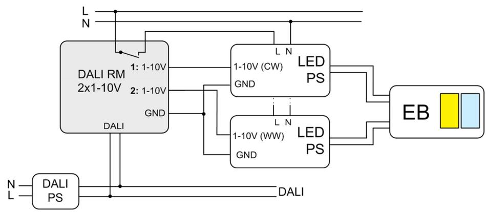
typical structure: control of two 1-10V LED-power supplies (one for CW, one for WW)
