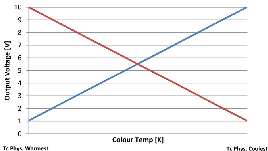
Hint: For a correct colour temperature the kelvin values of the used cold and warm luminaire should be entered as parameter TC PHYSICAL COOLEST and TC PHYSICAL WARMEST.
