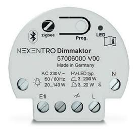
Universal dimming actuator for dimming of light e.g. for LED lights, high- and low-voltage halogen lamps in a Zigbee 3.0 system. It operates according to the leading edge phase control or trailing edge phase control principle and automatically sets the dimming principle suitable for the connected load. The device provides one input for connecting a push-button. Configuration and immediate function test via the Prog. button. It is installed in the appliance box behind the switch or push-button.
