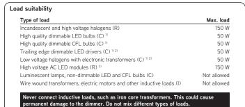
Dimming quality depends solely on the load electronics. Do not connect more than two LED or CFL bulbs to one CBU-TED. Do not mix different types of bulbs or loads.
